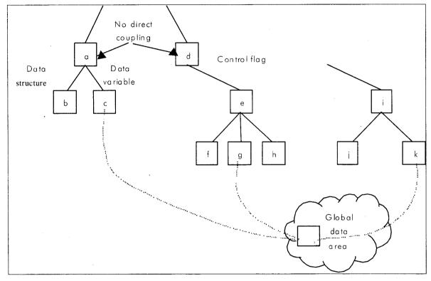
Figure 6.7: Types of Coupling
